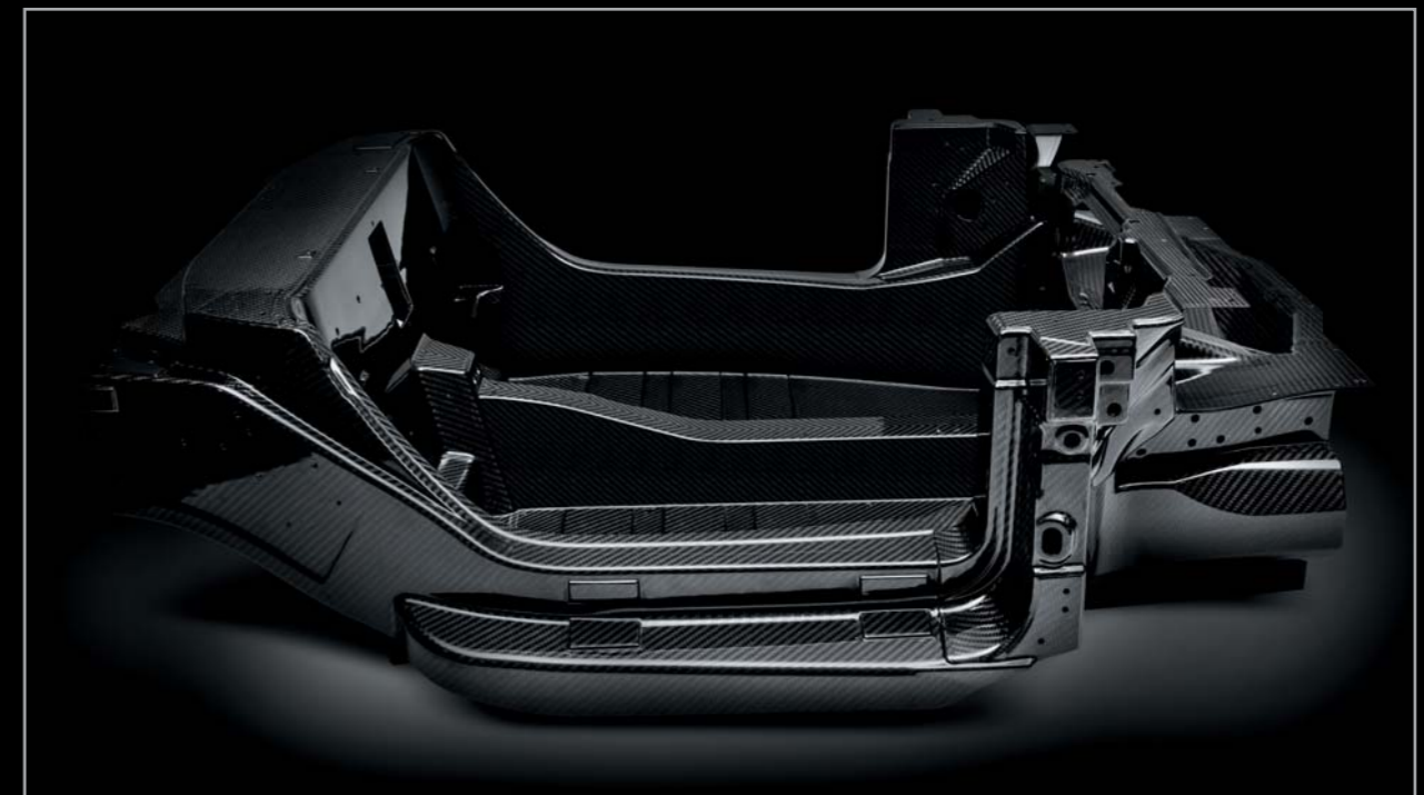
Carbon fibre monocoque chassis
