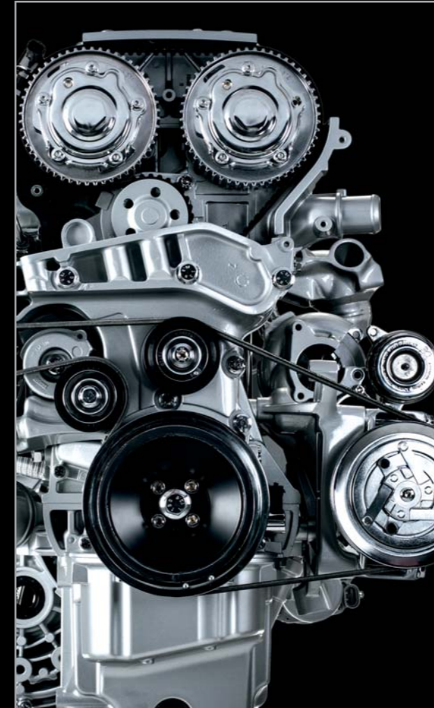
1750 cc, aluminium, 4 cylinder, turbocharged engine
