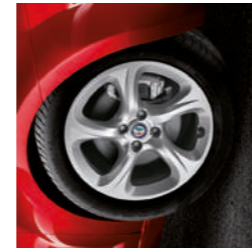
74B 16" 5-hole alloy wheels with 195/55 R16 tyres
