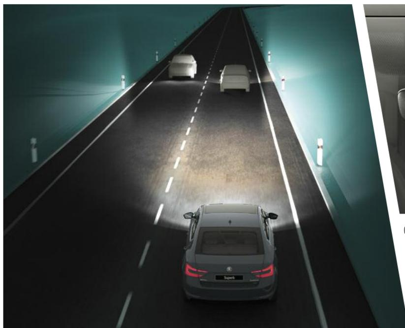
Now you can use high beam for longer without blinding incoming traffic. The Smart light assist can not only switch between the lighting functions but can also dim the high beam, using a multifunction camera located behind the rear-view mirror.
