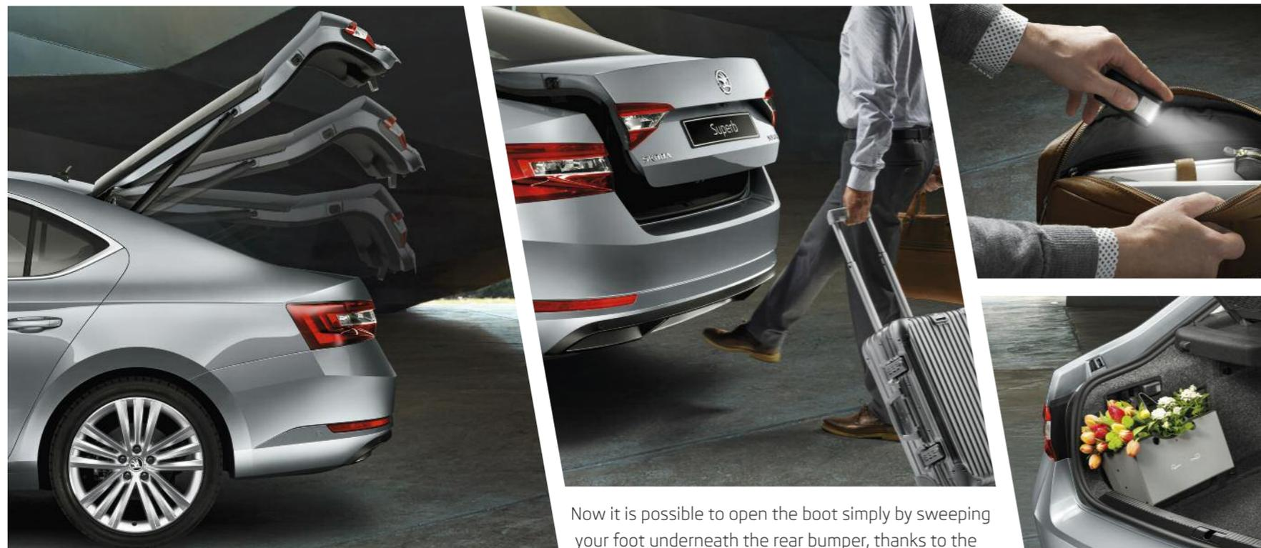
Now it is possible to open the boot simply by sweeping your foot underneath the rear bumper, thanks to the new Virtual Pedal. This feature enables contact-free access and is available with electrically-operated boot and KESSY (Keyless entry, start and exit system).
