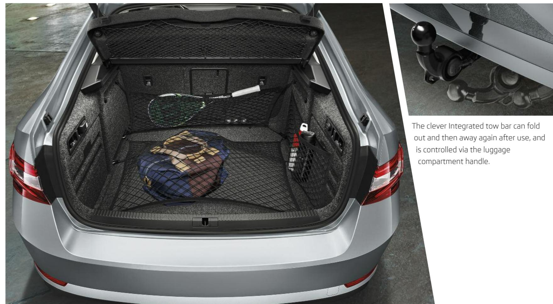
The clever Integrated tow bar can fold out and then away again after use, and is controlled via the luggage compartment handle.
