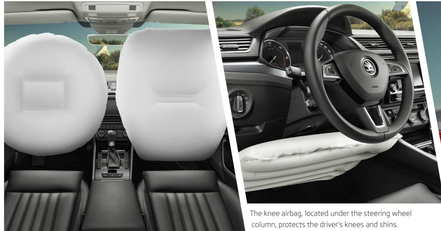
The knee airbag, located under the steering wheel column, protects the driver's knees and shins.
