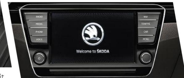
The Columbus navigation system offers comfortable touch control on an 8" colour TFT display. It has two SD card slots, a DVD drive and includes integrated Wi-Fi as well as SmartLink†.
