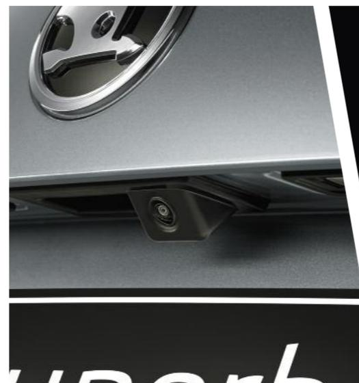
Enjoy easier parking by equipping your car with the Rear-view parking camera, which is located on the handle of the boot. It monitors the space behind the car and indicates the driving lanes, based on the vehicle width.
