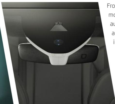
Other assistance systems that use the multifunction camera include Lane assist, for keeping the car in the right lane, and Travel assist for traffic sign recognition and display.
