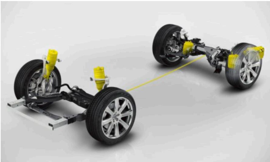
Choose the off road mode and the air suspension will raise the car by 40 millimetres. Hill Descent Control is activated at the same time: the car brakes for you on steep gradients – all you need to do is steer. The off road mode gets your XC90 to navigate challenging terrains – all you need to do is turn the elegant drive mode selector to the desired position.
