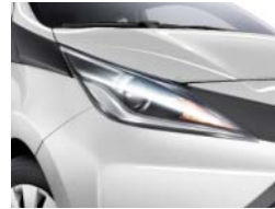
Projector headlights with LED tracer lights
