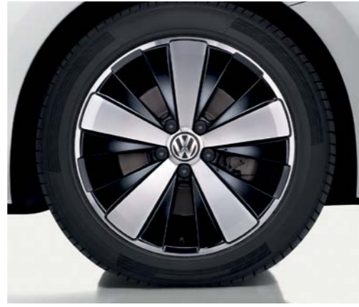
18 inch 'Twister' alloy wheels with 235/45 R18 tyres and anti-theft wheel bolts. SP D
