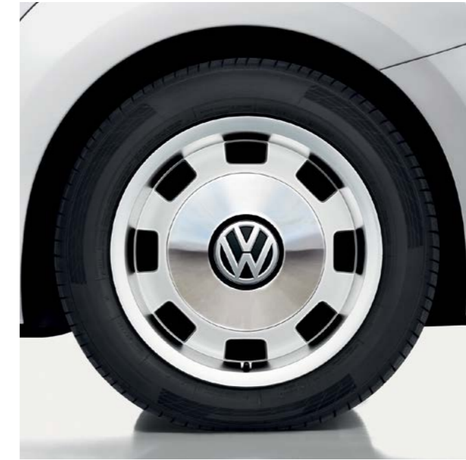
Design models feature retro 17 inch 'Orbit' alloy wheels with 215/55 R17 tyres, chrome effect rims and anti-theft wheel bolts.
