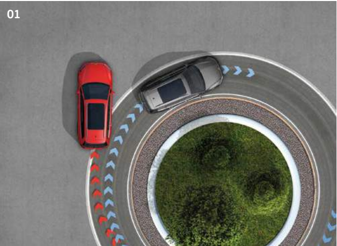
01 // XDS The Golf Estate features XDS, an extension of the well-known Electronic Differential Lock (EDL) function. This is linked to the Electronic Stability Control (ESC) hydraulics and works by applying pressure to the inner front wheel during fast cornering to prevent spinning. The one-sided, precise brake pressure helps to maximise traction, reduce understeer and improve responsiveness, thus making cornering even more sporty, safe and accurate. Standard on S, BlueMotion, SE, SE BlueMotion, GT and Alltrack models. XDSPlus is standard on GTD and R models.
