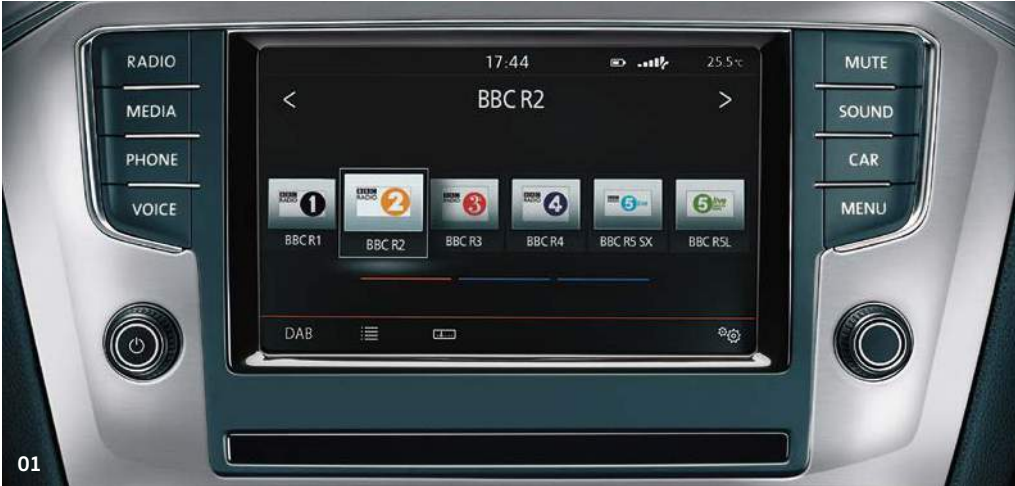
01 The Composition Media system is equipped with a 6.5 inch colour touch-screen with proximity sensor that recognises in advance your intention to touch the screen and automatically magnifies the display mode. Features also include DAB digital radio receiver, single CD player, MDI (Multi Device Interface) via USB connection for compatible products and SD card reader. The media system also includes Bluetooth telephone and audio connection for compatible devices 1 , simultaneous pairing of 2 compatible mobile devices, SMS functionality – allowing you to read, compose and send SMS messages using the touch-screen display to a compatible Android smartphone (while the vehicle is stationary), title and compatible cover art display and facilitates music playback from MP3, WMA and AAC files through eight speakers, front and rear. Finally, car information display and Think Blue. Trainer. – provide journey analysis and driver tips on your journey. Standard on S and BlueMotion models.
