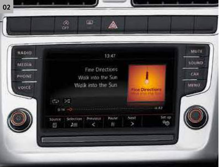
02 COMPOSITION MEDIA SYSTEM 6.5 inch colour touch-screen with proximity sensor, an MDI (Multi Device Interface) via USB connection for connectivity to an external multimedia source (compatible products only), title and cover art display, glovebox-mounted CD player and eight speakers. The media system also includes SMS functionality, allowing you to read, compose and send SMS messages using touch-screen display when your Polo is stationary (compatible Android smartphones only). The Think Blue. Trainer. – provides driver tips and journey analysis for more ecological driving and Bluetooth telephone and audio connection for two compatible devices 2 at the same time. Standard on SE models and above.
