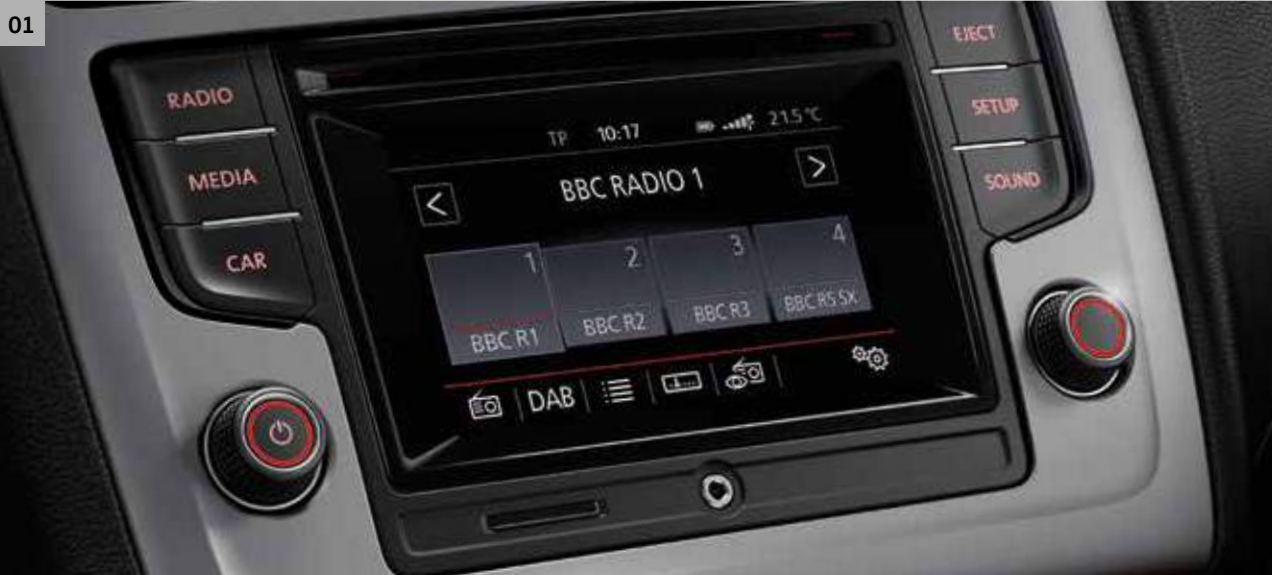
01 COMPOSITION COLOUR SYSTEM with 5 inch colour touch-screen, an AUX-in socket for connection to an external multimedia source, such as an iPod or MP3 player, a DAB digital radio receiver, dash-mounted single CD player, SD card reader, music playback from MP3, WMA and AAC files, USB connectivity 1 and six speakers. It also features Bluetooth telephone and audio connection for compatible devices 2 . Standard on S and S A/C models.
