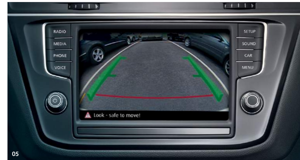
05 The rear-view camera , which forms part of the Park Assist and Trailer Assist options, is integrated behind the Volkswagen badge on the rear tailgate, displays the area behind your vehicle on the screen of the vehicle's audio system, helping you to manoeuvre into tight spaces quickly and easily. Auxiliary lines help you navigate safely into parking spaces, and thanks to the high resolution display, even small obstacles such as kerbs are visible. Optional on SE models and above.
