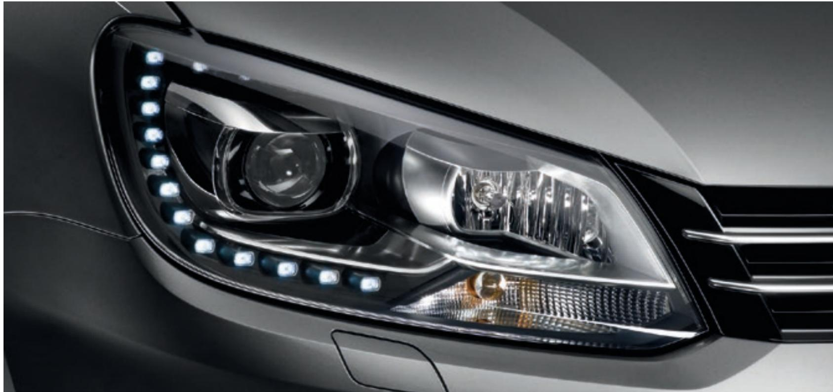
**S SE SP** **Bi-xenon headlights** feature automatic range adjustment, dynamic curve lighting and headlight washers to ensure the optimum headlight setting and illumination. Light distribution of the dipped beam is linked to speed, ensuring a longer beam is emitted at faster speeds for better illumination of the road ahead, while LED daytime running lights and LED rear number plate lights make sure your vehicle is more visible during the day. Model shown is Touran SE.
