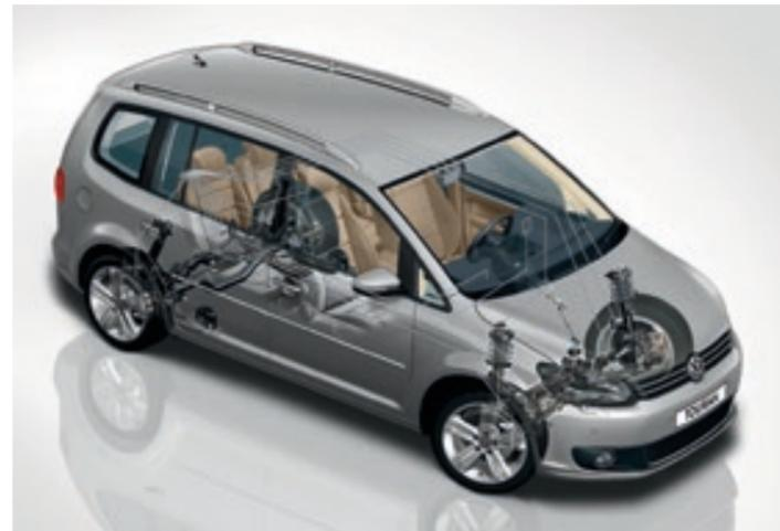
**SE SP Dynamic Chassis Control (DCC)** adapts the damping control and shock absorption rate to the road conditions and driving style you require within milliseconds. At the touch of a button, you decide how firm or comfortable you wish to set the suspension, with a choice of three settings: Sport, Comfort or Normal. In Sport mode, the steering also adapts to a sporty driving style. Not available on BlueMotion Technology models.
