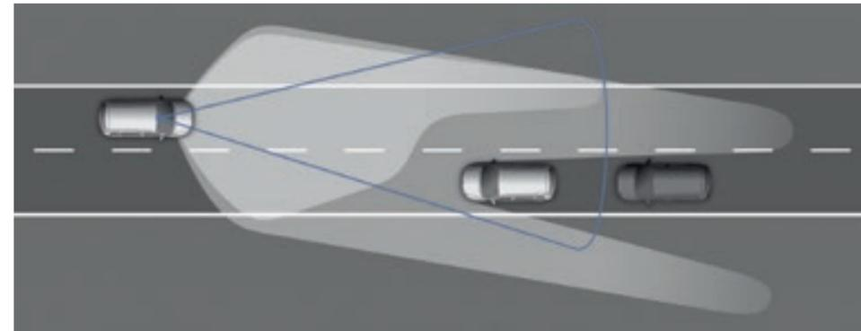
**S SE SP** The **High beam assist** function ingeniously senses the lights from oncoming vehicles and switches between main and dipped beam accordingly.
