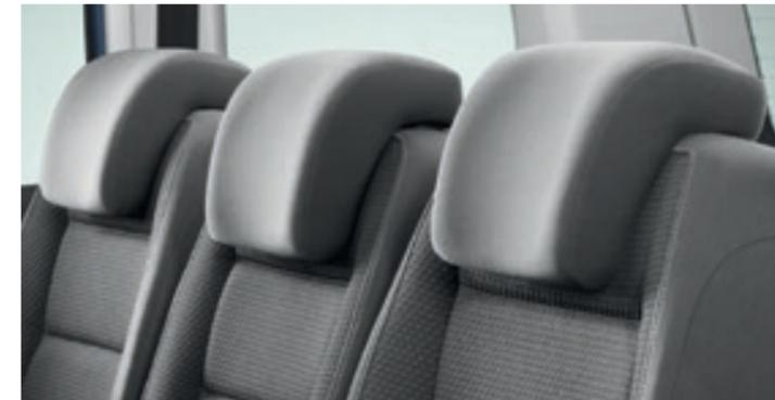
**S SE SP** In the 2nd row, all three single seats are equipped with **head restraints and three-point automatic seat belts**, and the outer seats are fitted with height adjustable seat belts.
