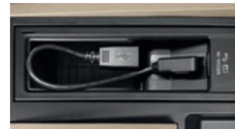
**SE SP** The Multi Device Interface (MDI) with USB and iPod cables enables you to connect and charge a compatible device, while track selection is viewed and selected via the vehicle's radio system.
