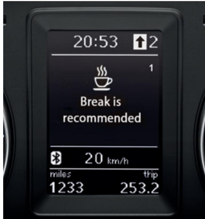
**SP** The **Driver Alert** system detects when the driver is becoming tired and recommends taking a break. This is achieved by monitoring driving behaviour closely, noting any erratic steering wheel movement and alerting the driver via visual and audible warnings.
