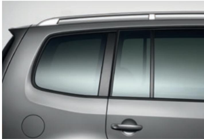
SE SP The heat insulated rear tinted glass from the B pillar backwards reduces the glare of sunlight by up to 65%, ensuring a pleasant interior temperature in the passenger compartment and giving occupants additional privacy.
