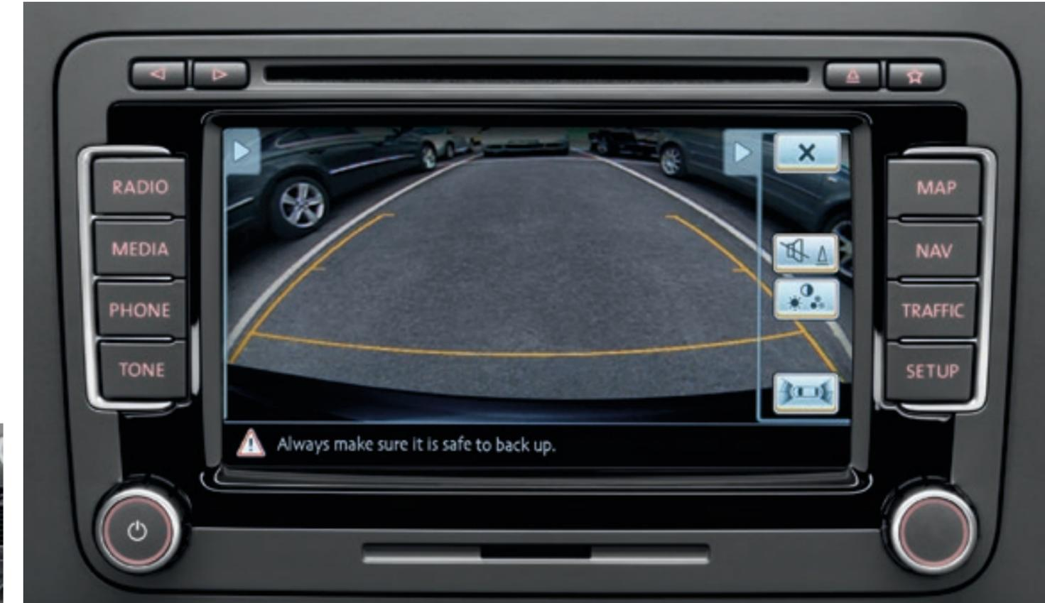
ⓂⓈ ⓂⓈ The rear-view camera, shown here as part of the RNS 510 touch-screen DVD navigation/DAB radio system option, is located in the rear tailgate and reproduces an electronically straightened image on the audio system's display. This provides an unobscured view to the rear of the vehicle, making parking easier and safer, even when towing a trailer.
