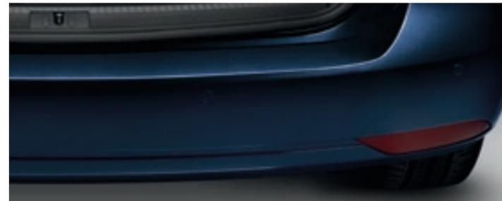
Ⓢ ⓂⓈ ⓈP Rear parking sensors, are ultrasonic, audible with audio volume reduction when activated and optical parking display via vehicle's audio system.
