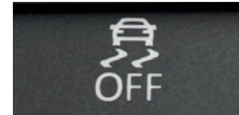
**S SE SP** The **Electronic Stability Control (ESC)** utilises sensors to detect critical situations at an early stage, reacting within milliseconds by controlling the speed of individual wheels, helping to bring the vehicle under control.
