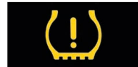
**S SE SP** In the event of a change in air pressure, the **tyre pressure loss indicator** symbol appears in the multifunction display, advising the driver to rectify the situation.
