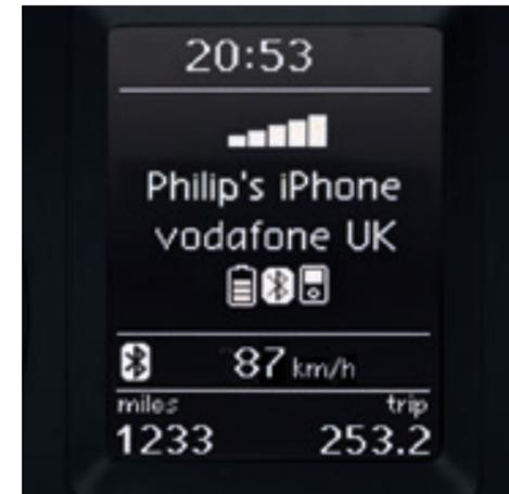
**SE SP** Bluetooth telephone connection for HFP (Hands Free Profile) enabled telephones allows you to use your phone safely whilst driving. The phone book and call information is displayed on the audio system's display and on the multifunction computer.
