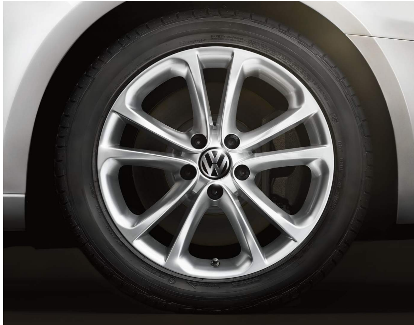
CC 'SPA' 7 1/2" x 17" alloy wheels with 235/45 R17 self-sealing tyres and anti-theft wheel bolts.
